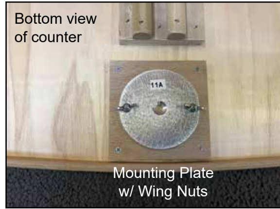
1) Mounting plate & wing nuts, in packed position.
